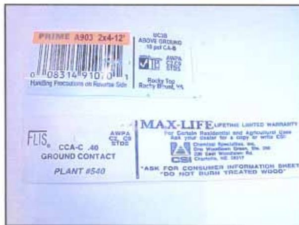
Figure 1. Example tags from CCA and CA-B treated lumber which are both greenish in color, but the important issue for contractors and owners is level of protection against decay. It is based on the specific chemical used and minimum retention per AWP standards. The chemical and retention can be found in small print on the quality tag attached to the end of each piece.
