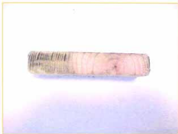
Figure 2. The heartwood section of this 5/4x6 southern pine deck board is clearly indicated by the color differentiation. The heartwood section containing the pith is mostly untreated as evidenced by the yellowish pine color. The sapwood section is well treated with the greenish preservative.
