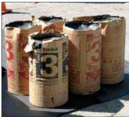
Figure 6. Different types of asphalt have different softening points. The type 3 material shown here softens at about 200°F but is applied at over 400°F.
