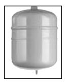
A WaterGuard Expansion Tank eliminate these problems, by giving water a place to go when thermal expansion occurs. When a water heating cycle ends, or when any fixture is opened within the system, the impact of thermal expansion is reduced, and water drains out of the expansion tank back into the system.
