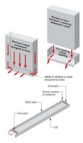
Obviously, the lower lip on the pan flashing would be angled out and over your angled brick and not vertical like the drawing above.
