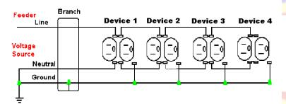
By testing receptacle in sequence from furthest from the panel to closest with a load test, hidden defects can be identified and corrected
