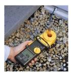
A ground resistance clamp meter enables electricians to measure the resistance of the ground electrode in a fraction of the time required using the traditional three-point fall of potential test.
