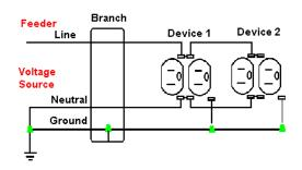
The grounding circuit must not rely on any device to maintain the circuit. The NEC requires that the removal of any device cannot interrupt the ground path
